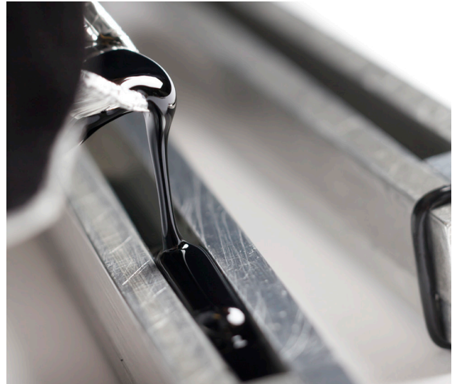
Figure 4: Preparation of BBR test specimen
